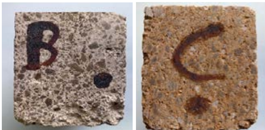
Figure 1. (Left) VIMAG SP 86 B with no cracks. (Right) Magnesia spinel brick with no cracks.
